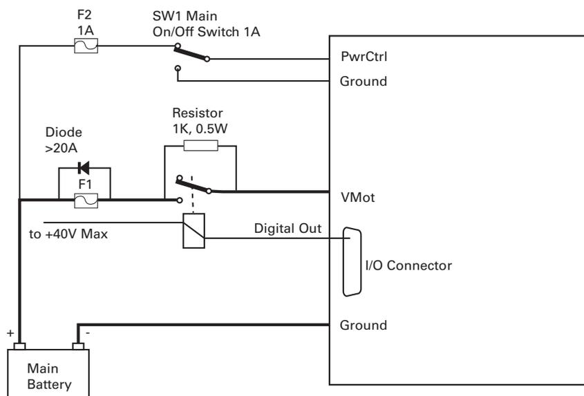
FIGURE 9. Contactor wiring diagram
