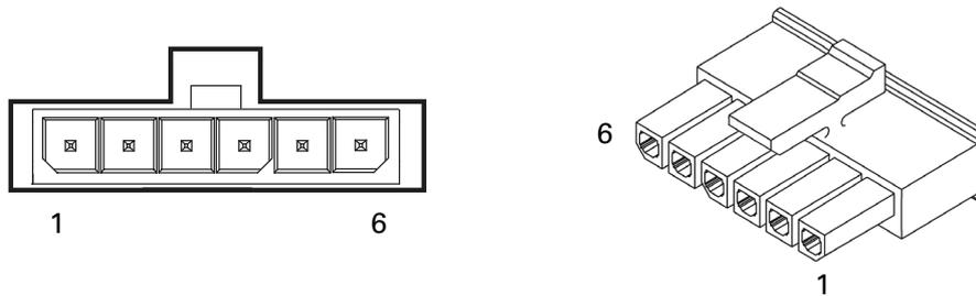
FIGURE 11. Encoder connector
