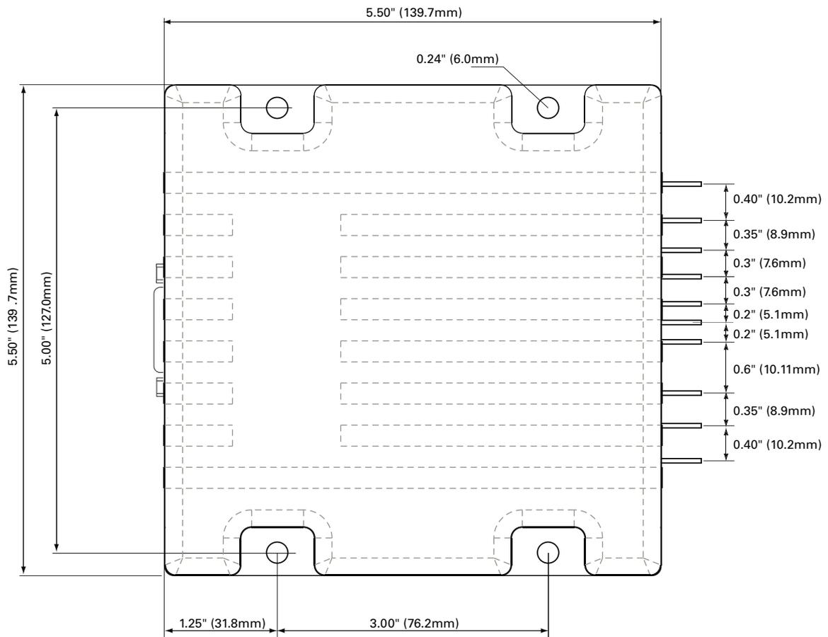
FIGURE 17. MDC2xxx top view and dimensions
