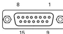
FIGURE 12. Connector pin locations
