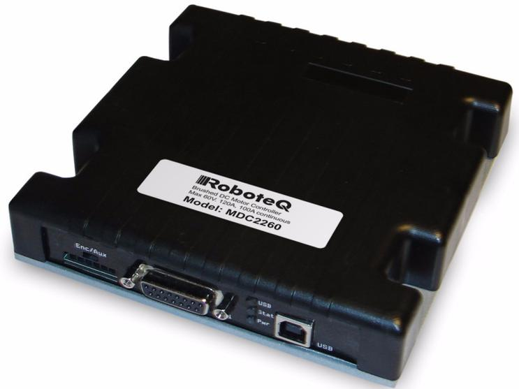
Roboteq's MDC2xxx controller is designed to convert commands received from an RC radio, Analog Joystick, wireless modem, PC (via RS232 or USB) or microcomputer into high voltage and high current output for driving one or two DC motors. Designed for maximal ease-of-use, it is delivered with all necessary cables and hardware, and is ready to use in minutes. Using CAN bus, up to 127 controllers can be networked at up to 1Mbit/s on a single twisted pair.
