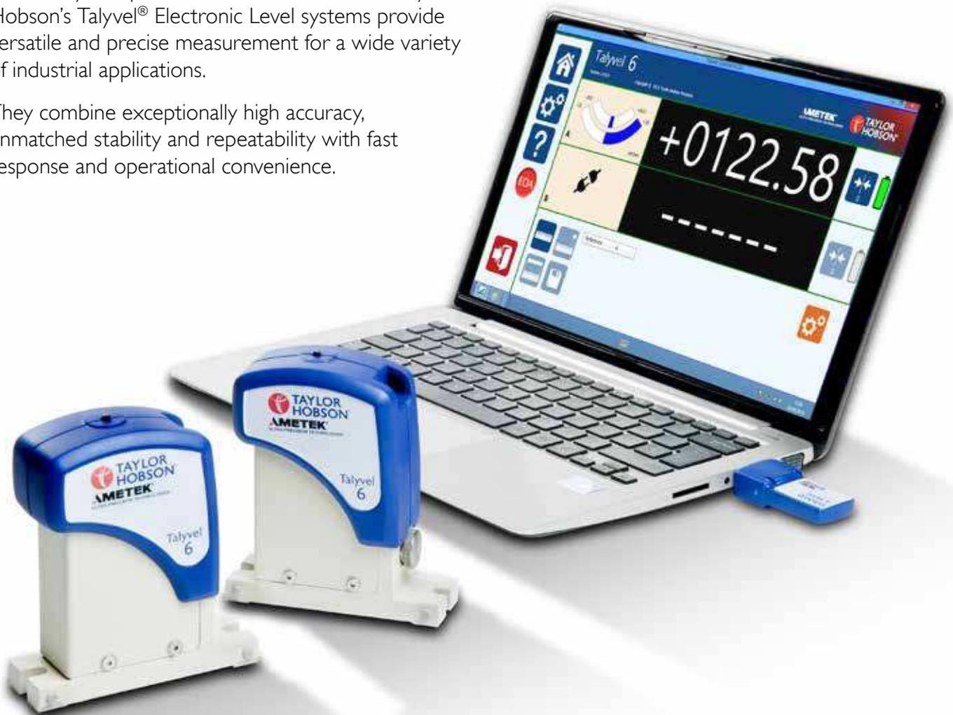
Incorporating a compact, highly stable, pendulum transducer in the Level Unit and interfacing directly to a tablet PC or laptop with dedicated software, Talyvel® 6 provides rapid and simple reading of angle of tilt and measurement relative to gravity. It is simple to calibrate and operate, with a fast measurement response time.
