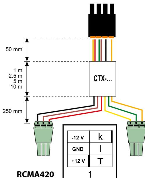
Connection to the RCMA420 residual current monitor using the CTX... connecting cable.
