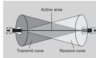
large field of view, they can be easily aligned even at distances of 40 meters. Simultaneously they are insensitive to shock and vibrations and the resolution of the misalignment.
