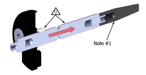
Note #1 - Shaft fitting tool included in spares kit DXK-4 This must be used when re-fitting centre shaft
