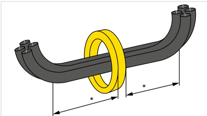
\* Distance to the 90° angle = 2 x transformer outside diameter
