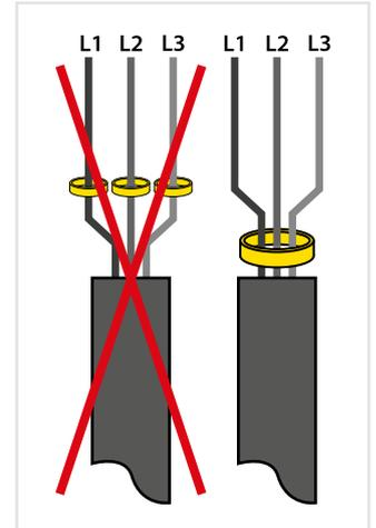
Make sure that all current-carrying leads are passed through the measuring current transformer
