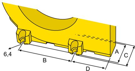
Snap-on mounting on DIN rail: for vertical or horizontal mounting: W20, W35, W60 und W20-8000, W35-8000, W60-8000
