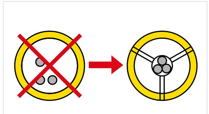
The leads must be aligned with the centre of the measuring current transformer
