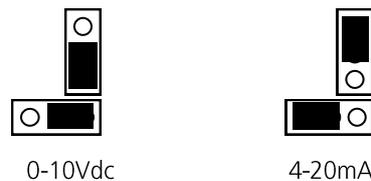
If the range links are incorrectly set, or missing the output range
