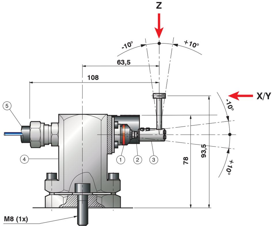
The probe is usually fixed to a holder, on the machine table beside the working area.
