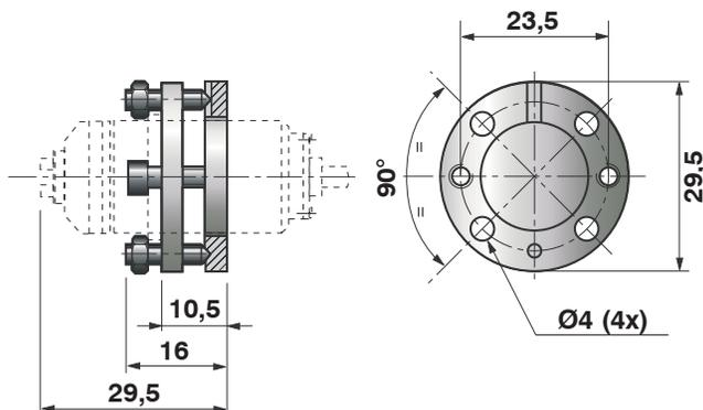
The holder is fastened to the machine by means of the four fixing screws. By acting on two couples of screws, it is possible to pivot the holder and allow the probe adjustment.
