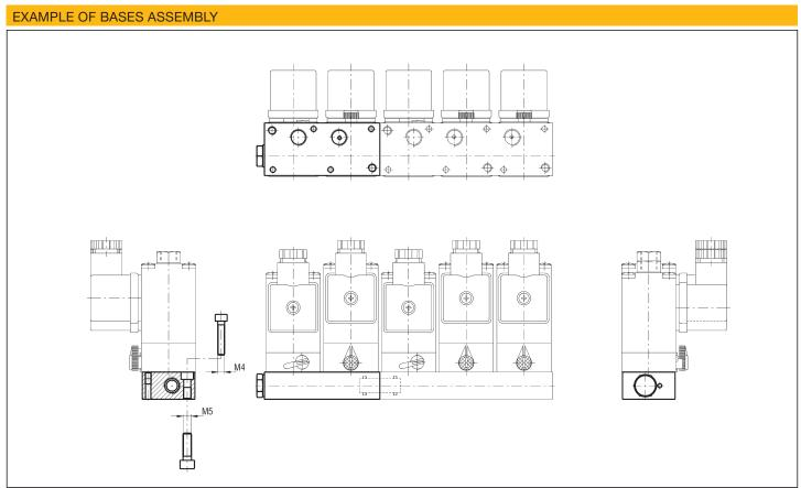
P.S.: The connection nipple is supplied as standard with the multi-station base
