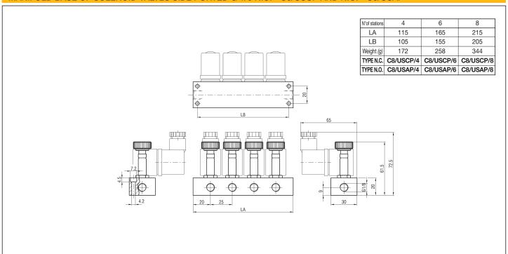
$\hbox{P.S.: MANIFOLD BASES OF SOLENOID VALVES WITH "MIXED" OPERATION (N.O./N.C.) ARE SUPPLIED UPON REQUEST}$
