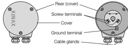
Fig. 3. Screw terminals / screwed cable gland
