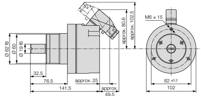
Fig. 4. KINAX WT 707 with plug connector.
