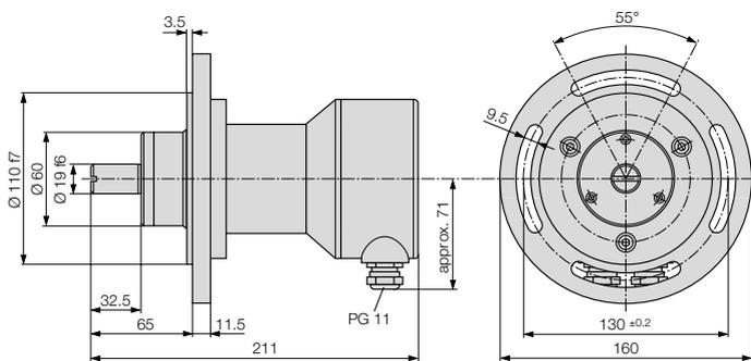
Fig. 15. KINAX WT 707 with additional gear, screw terminals, cable glands and flange.
