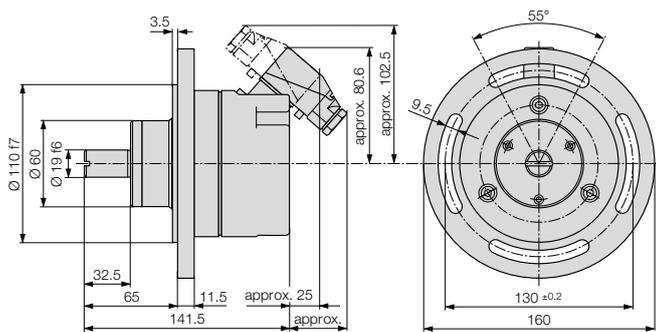
Fig. 12. KINAX WT 707 with plug connector and flange.
