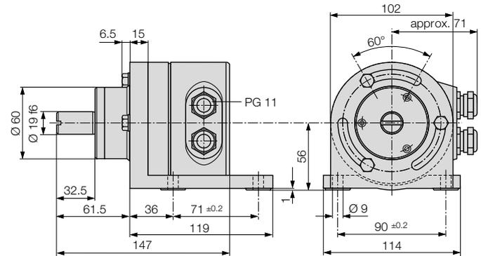
Fig. 9. KINAX WT 707 with screw terminals, cable glands and foot.
