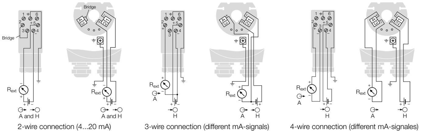
4-wire connection with electrical isolation (different mA-signals)
