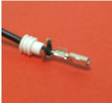
Photograph CK1102, showing some partly crimped flaps
