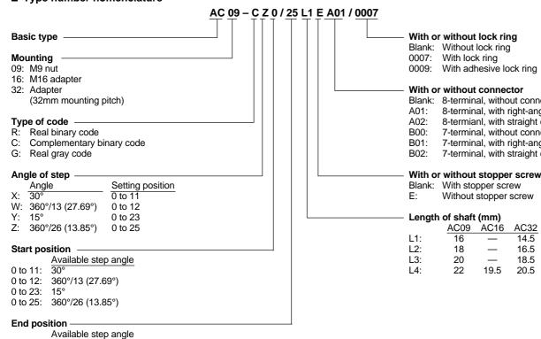
0009: With adhesive lock ring With or without connector Blank: 8-terminal, without connector 8-terminal, with right-angle connector 8-termianl, with straight connector 7-terminal, without connector
