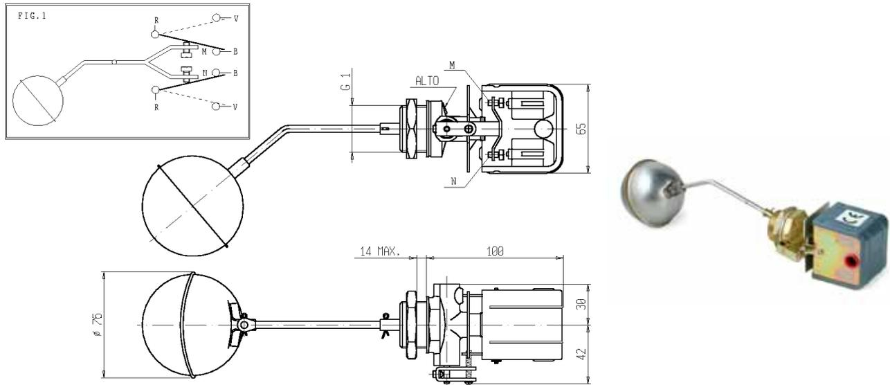
**FEATURES** - Device designed to control the water level into pressurized or non-pressurized tanks. Fitted by two electric deviation switches, fast and non-vibration type with silver-plated contacts: one operating on the minimum level and the other one on the maximum level.
