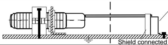
The end of the cable must be connected outside the hazardous locations. Reliable, noncorrosive holding of the protection earth connection.
