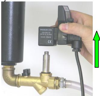
4. Unscrew the valve top nut using a 14 mm wrench.
