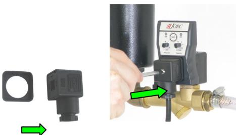
8. Remove the protection cap from the connector and connect your power cable to the connector as shown below.
