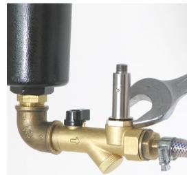
*Do not use the valve shaft as a lever!*
