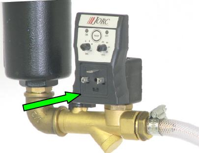
9. Place the connector gasket on the connector, plug the connector on the timer as illustrated below and tighten the screw (max. torque 1Nm). Make sure both gaskets are secured properly to ensure IP65 rating.
