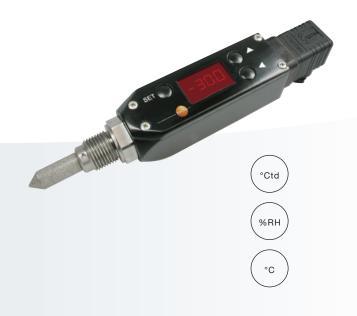
The testo 6740 was especially developed for trace humidity measurement in compressed or dry air (e. g. granulate dryers). Thanks to a special adjustment, optimum accuracy in the trace humidity range has been achieved.
