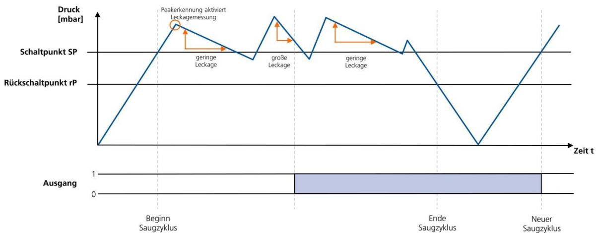
Another application for condition monitoring mode occurs if the regulation threshold of the vacuum system is never achieved and the vacuum generator permanently drains. In this case, if the end vacuum is 20 mbar lower than the start vacuum, the switching point will also be activated.
