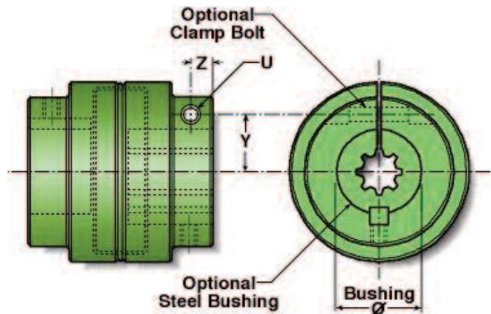
**Magnaloy Coupling's** full range of flexible inserts permit custom design performance for a wide range of applications. All insert materials offer complete electrical insulation, as Magnaloy's design eliminates all metal-to-metal contact.
