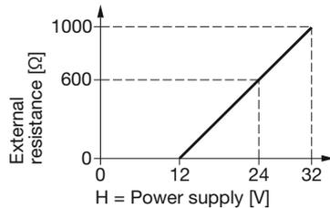
$$R_{\text{ext max.}} [\text{k}\Omega] = \frac{H [\text{V}] - 12 \text{ V}}{20 \text{ mA}}$$
