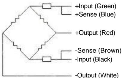
The two "sense" wires sample the bridge supply voltage at the load cell. Complete compensation of change in the lead wire resistance, due to temperature change and/or cable extension, is achieved by feeding this voltage into appropriate electronics.
