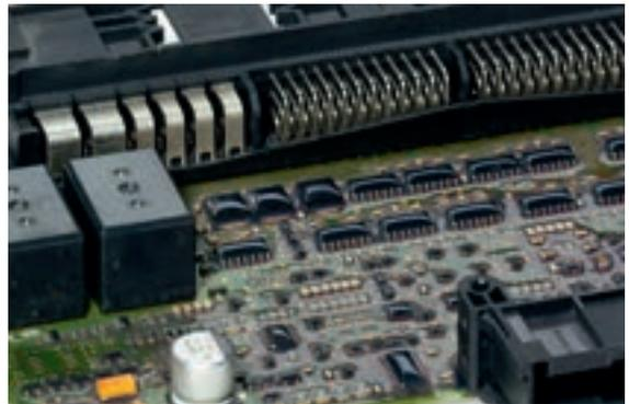
BECTRON® Thin Film Coatings are suitable for many process methods including select coat, spray, dip and selective flooding. Examples of applications include PCBs for the automotive and marine navigation industries, PCBs for industrial electronics, hybrid circuits, SMD assemblies and other discrete electronic components.
