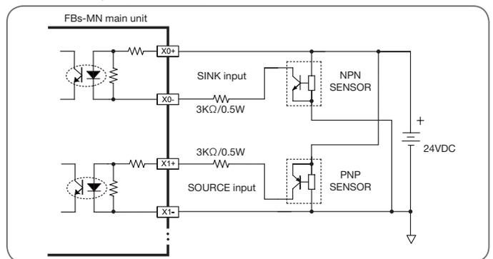
Wiring of 24VDC single-end SINK input
