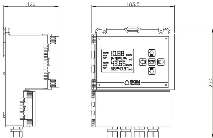
**VLW90M****Level, open channels flow and pumps control unit**
