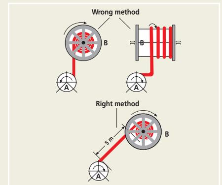
Figure 3. Transfer of cable from original delivery drum A to the cable winding reel B.
