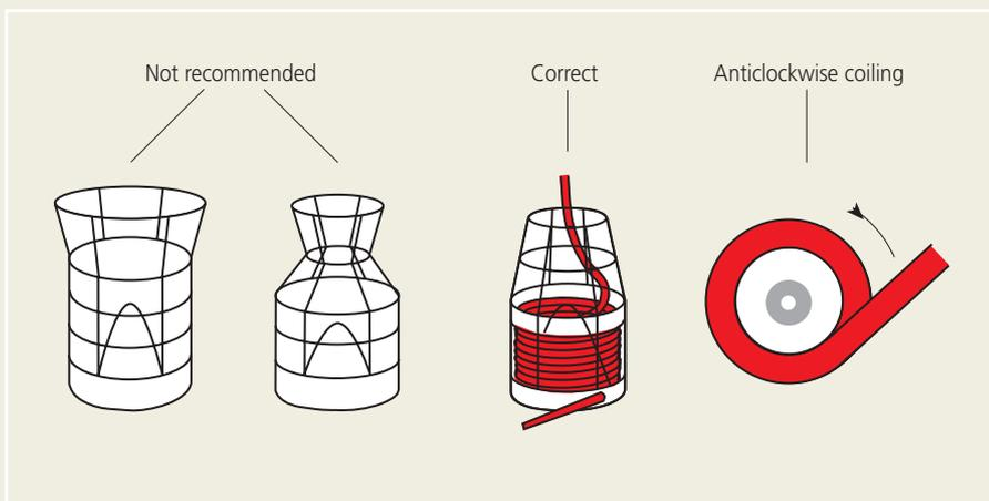
Figure 1. Shape of the basket and direction of coiling.
