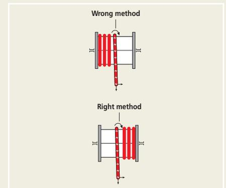
Figure 4. Winding of cable onto multi-spiral reel.
