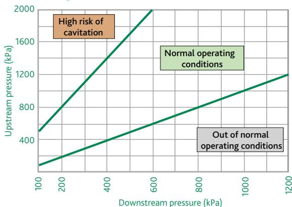
In order to minimise the risk of cavitation in the reducing valve, which could cause malfunctions with the risk of erosion in the seal area, vibration and noise, you are strongly advised to refer to the operating conditions specified in the diagram.
