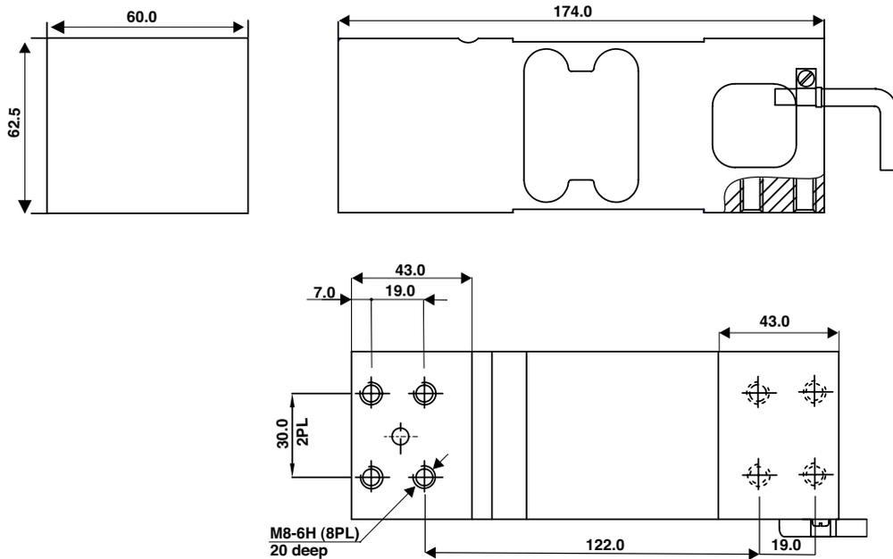
Aluminum High Capacity Single-Point Load Cell
