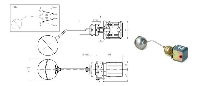
**FEATURES** - Device designed to control the water level into pressurized or non-pressurized tanks. Fitted by two electric deviation switches, fast and non-vibration type with silver-plated contacts: one operating on the minimum level and the other one on the maximum level.
