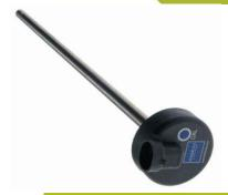
The **Model T/LL130** series is designed for use in water, coolant or fuel/oil tanks and provides a factory set variable resistive, voltage or PWM (Pulse Width Modulated) output suitable for driving industry standard fuel gauges or connecting into PLCs.
