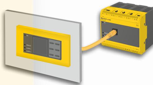
The display unit FP200 is mounted in the front using retaining clips and connected via a provided RJ45 connection cable to the basic devices without display. This installation variant makes it possible to install the display of the device in the control cabinet front without having to route the system connection with up to 1,000 V.
