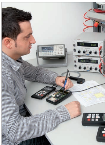
Acceptance test of a crack depth gauge
