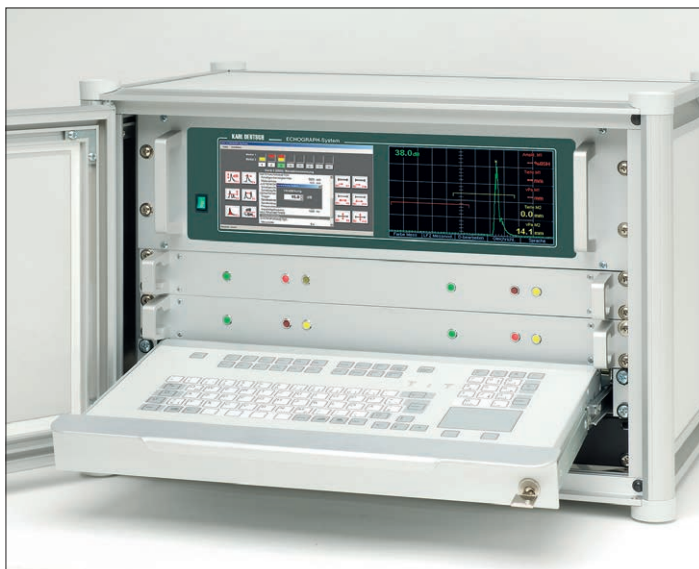
ECHOGRAPH 1093 - Digital ultrasonic instrument with up to 8 channels
