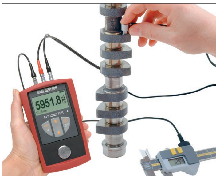
ECHOMETER 1076: Sound velocity measurement on a camshaft
