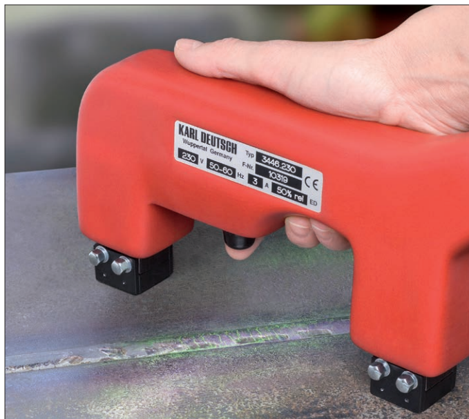
Handheld yoke for weld inspection (DEUTROPULS 3446)
