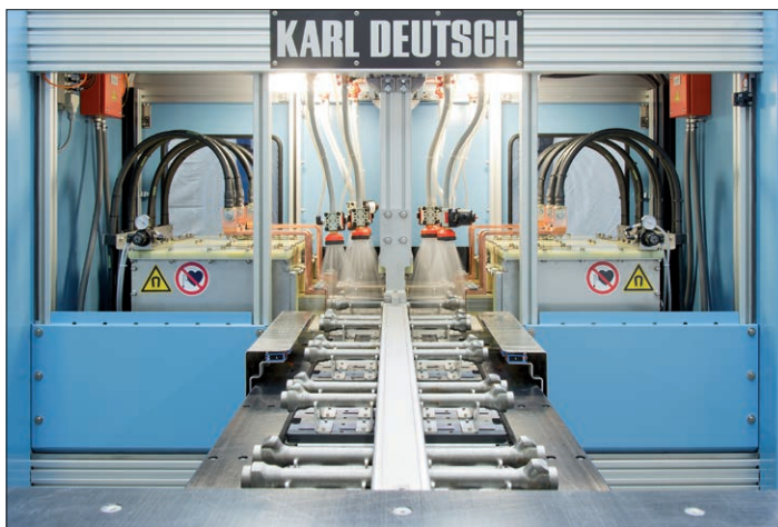
DEUTROMAT with chain conveyor, 8 components per cycle
