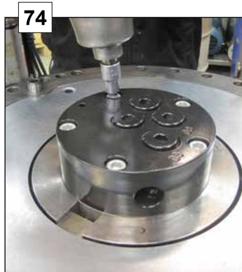
**WARNING!** If the rotator is normally positioned the transmission can fall down if the bottom plate is loosened!
