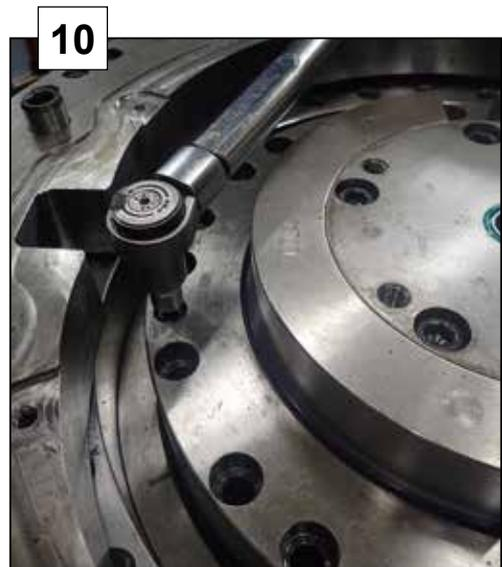
Remove stator plate lower.
