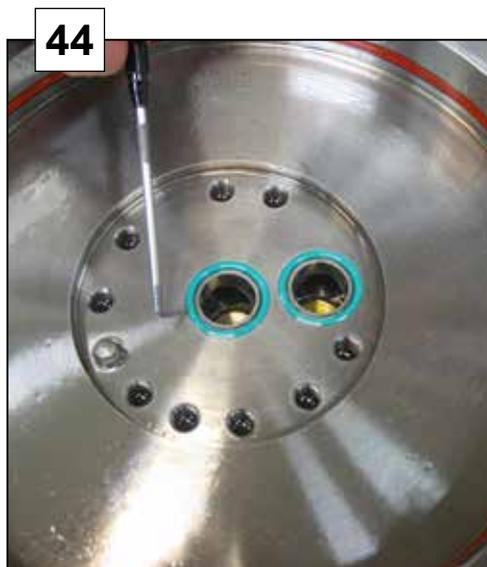
Assemble the block upper in the stator upper.
