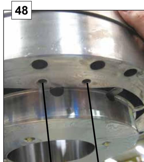
Note the positions of the rotation channels in the stator upper.
