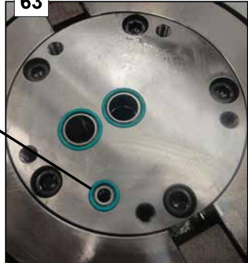
If needed grease the recesses for the transmission in the lower link.
