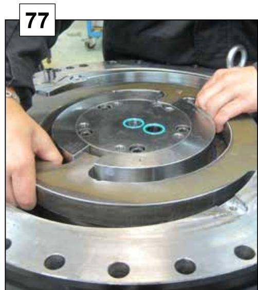
Remove 3 pcs of M8x50 screws in the lower link.
