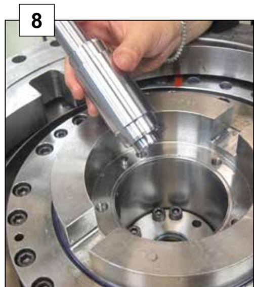
Remove 20 pcs of M12x110 screws to loosen the motor part.
