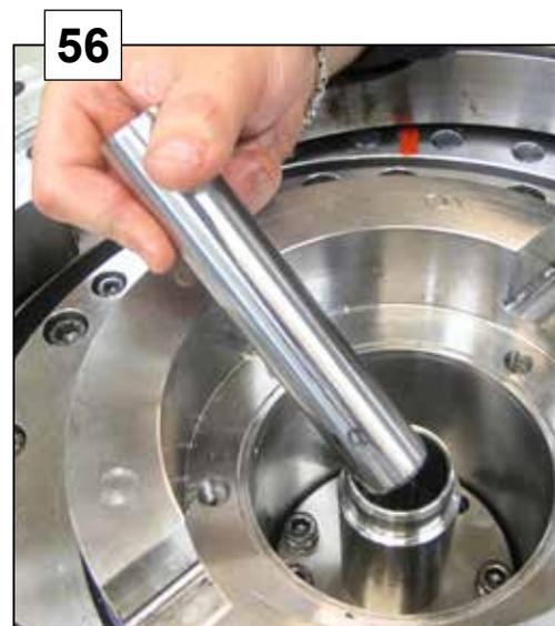
Grease the edges of the outer tube and the internal tube.
