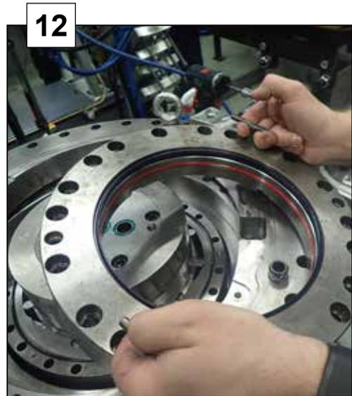
If needed remove the wiper seal (only if it has a damage).
