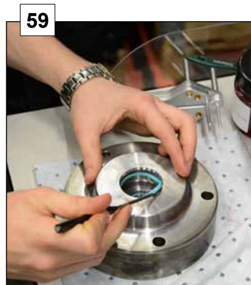
Make a mark on the outside of the rotator shaft and the block lower where the dowel pins are positioned.
