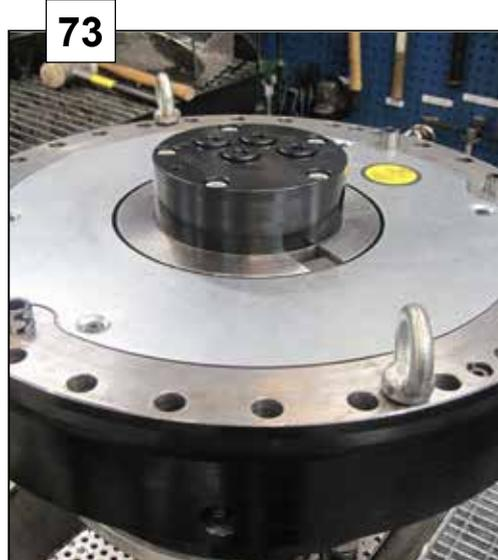
Remove the manifold block by loosen 5 pcs of M12 screws.
