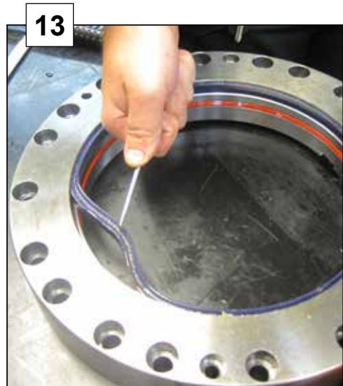
Remove the seal in stator plate lower.
