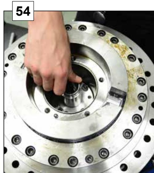
Grease the internal tube.
