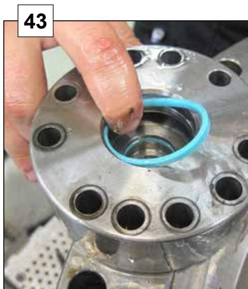
Remove 2 pcs of o-rings at the grapple channels in stator upper.
