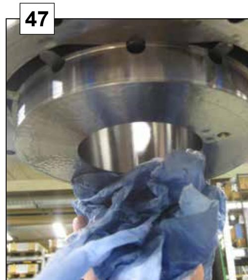
Note the positions of the rotation channels in the stator frame.
