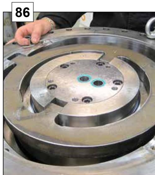
Assemble the bottom plate with 4 pcs of M8x12 screws
