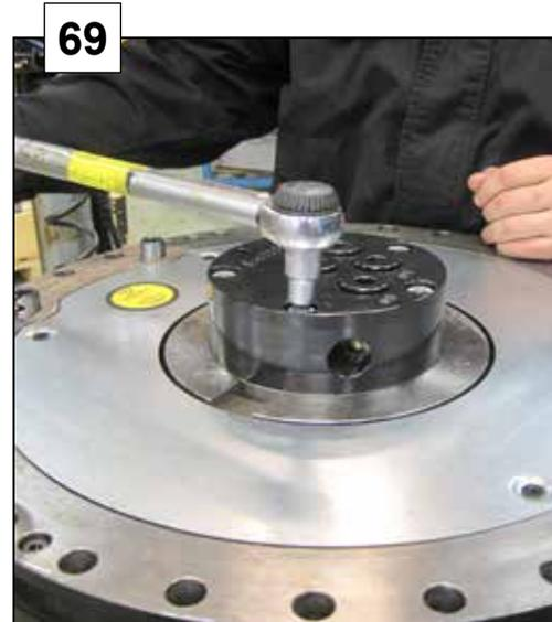
Test of the rotator function.
