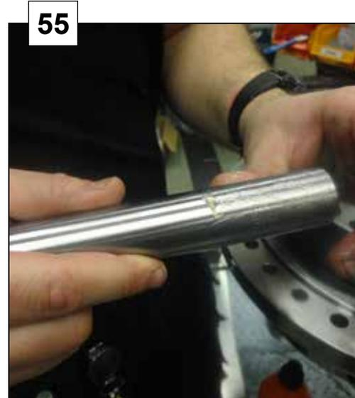
Assemble the internal tube inside of the outer tube.
