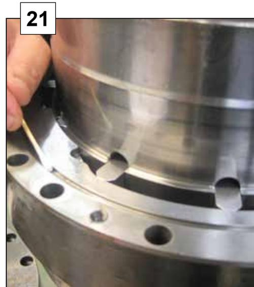
Lubricate the seal seat with oil.
