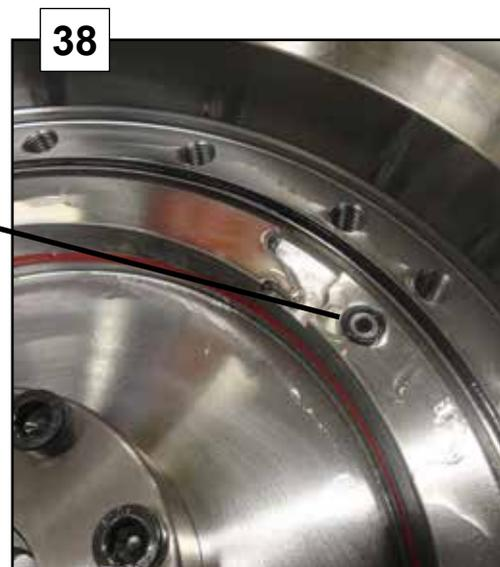
Clean stator upper from oil to make the assembly of the motor possible.
