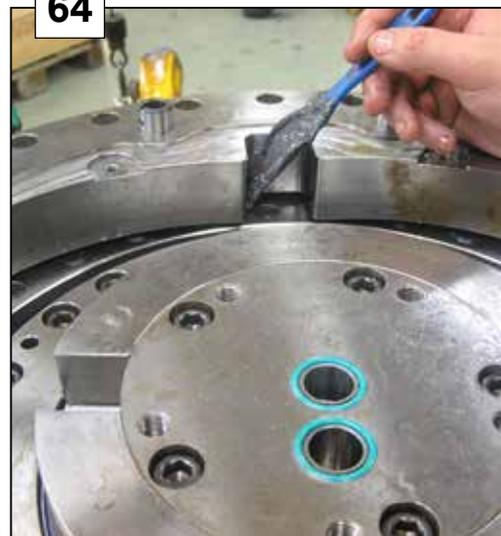
Grease the recesses for the transmission on the rotator shaft.
