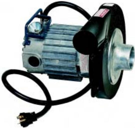
Known for durability and high production, our blower is designed with a hard coated fan and a steel chamber, powered by a rugged Dumore motor with manual thermal overload protection. This blower is designed to blow cellulose insulation fibers that are properly conditioned by agitation in the hopper. The high speed (13,000 r.p.m.) conditioning effect of the blower fan provides unsurpassed performance in sidewall blowing and coverage in open attic blowing.
