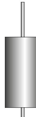
On request the float can be supplied with through hole and therefore be positioned in the required position without having to cut the rod (which can therefore be as long as the height of the tank). If necessary, the liquid control point can be subsequently be modified as required by simply moving the float. Available on request with AISI 316 stop.
