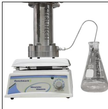
Photo 13: Permeate Collection Vessel And Stirring Plate
