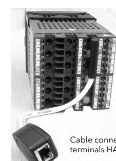
Cable connected to terminals HA to HF
