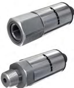
The PT1 pressure transmitters operate with ceramic measuring cells. They are cylindrically shaped, made of stainless steel and have no display. Depending on the type, the processed signal is output as 4...20 mA (2-wire) or 0...10 V (3-wire).
