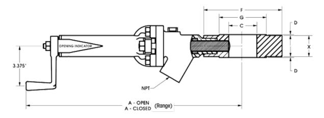
For use with Ram-Type Drain Valves a recess is required. Use piloting dimensions as discussed on page 10.
