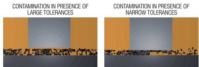
Solid contamination mainly causes surface damage and component wear.
