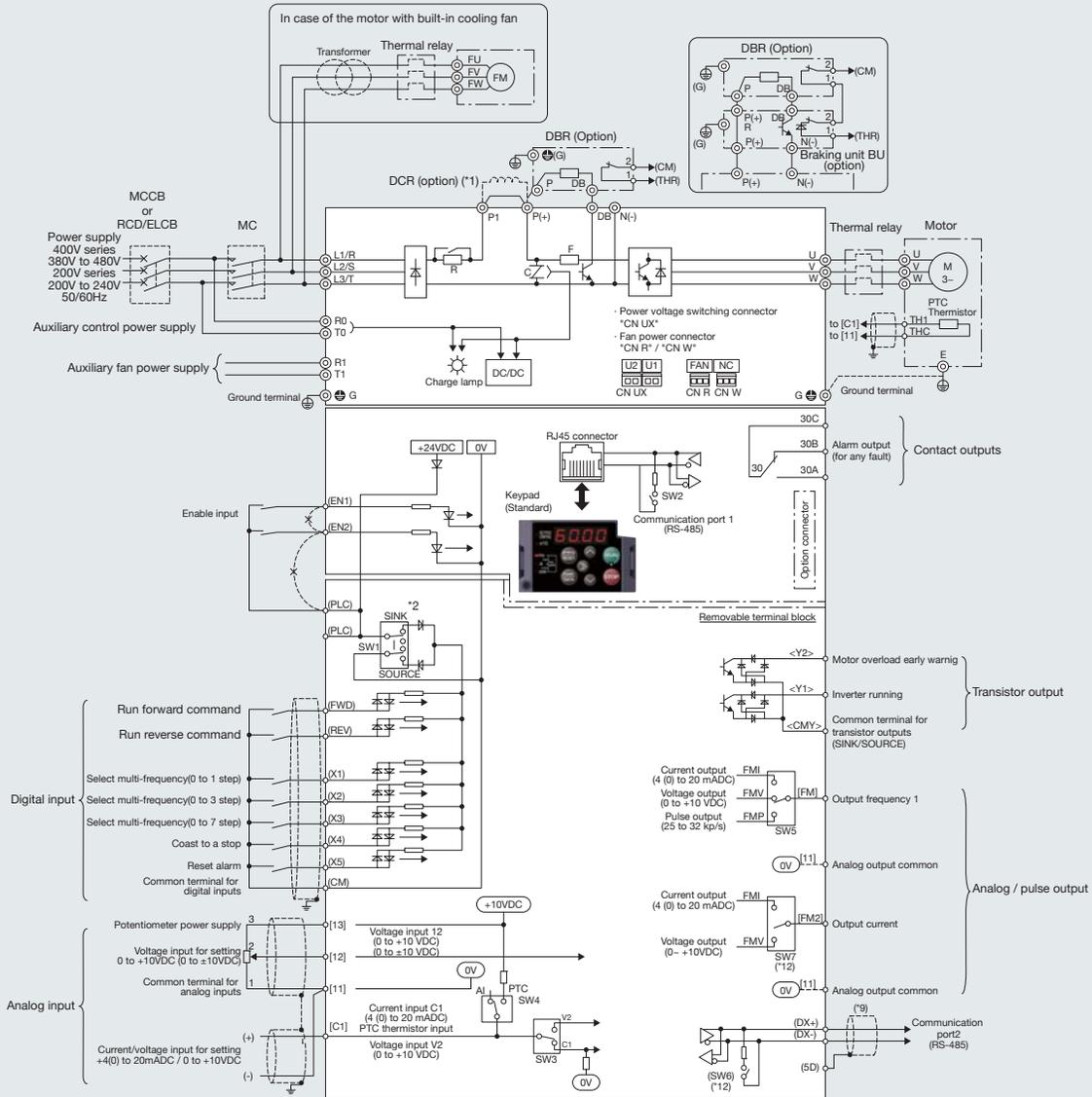
DBR: Dynamic Braking Resistor
