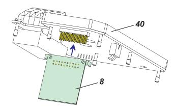
One module "Additional inputs / outputs" **8** can be plugged onto main electronics **40**:
