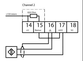
V Electromagnetic Transducer
