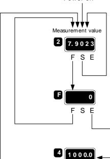
After connecting the power the standard measurement mode as selected in the configuration is displayed
