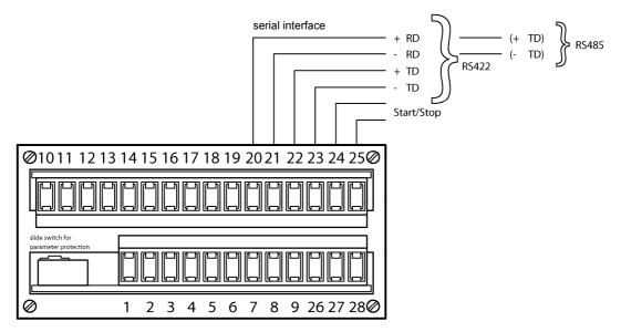
Terminals 20 -23 are used for the serial interface or analog output
