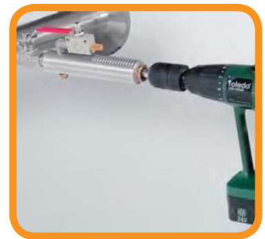
Drilling under pressure
