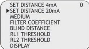
Use and to modify that value; in the Fig.25 example, the 20mA distance is 500mm. Press to confirm.
