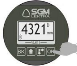
Select the parameters by moving the cursor with , and confirm with ; press to exit
