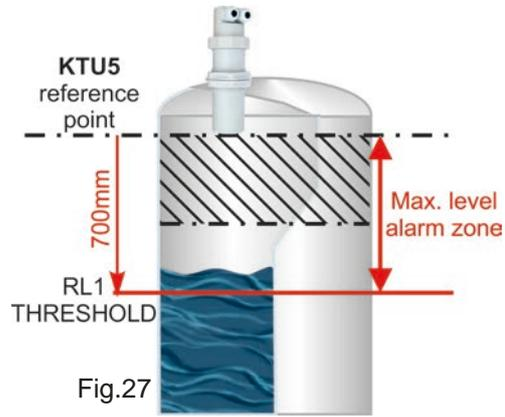
When confirming with the **ENTER** button the maximum level threshold value storage, in the example 700m (figures 29 and 30), the **KTU5** activates RL1 with the following default settings for level alarm threshold:
