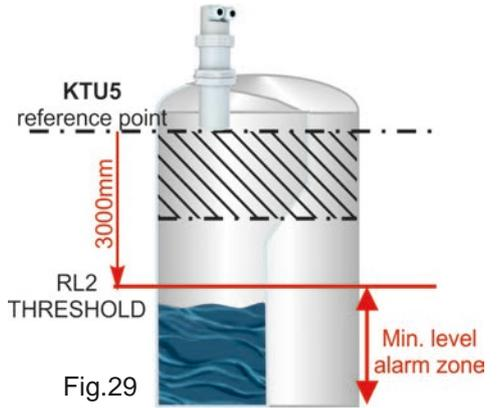
When confirming with the **ENTER** button the maximum level threshold value storage, in the example 3000mm (figures 31 and 32), the **KTU5** activates RL2 with the following default settings for level alarm threshold:
