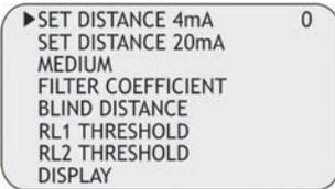
Use and to modify that value; in the Fig.25 example, the 4mA distance is 3500mm. Press to confirm.
