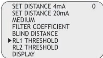
Use **DOWN** and **UP** to modify the value; in the Fig.29 example the RL1 max. level threshold distance is 700mm.
