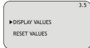
Displays the max. and min. distance measured from power on.
