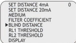
Use and to modify the value. Press to confirm. The minimum value is 250mm (5m max vers.) or 400mm (8m max vers.).
