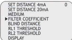
Use and to modify the value. Input a value from 1 to 99. Press to confirm. In fig.27 value choice example.
