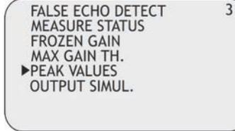
The system store the maximum distance and the minimum distance measured since the power is turned ON.
