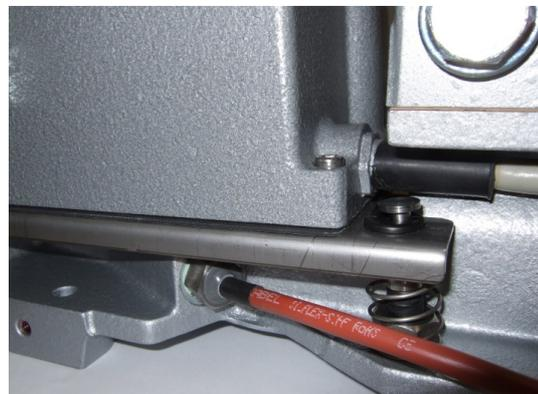
**Figure 3:** Base plate heating element.
