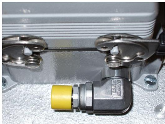
**Figure 5:** Main connector with heater removed and plug capped off.
