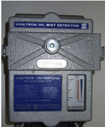
**Figure 1:** Measuring Head of VN87plus series.
