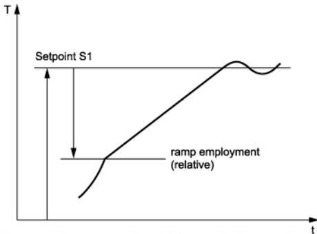
The main setpoint S1 and the point of ramp employment are linked as difference with one another. This difference can take positive or negative values, i.e. starting point for the ramp can be above the setpoint at cooling function or below the setpoint at heating function, and automatically runs along with adjustments of the desired value.
