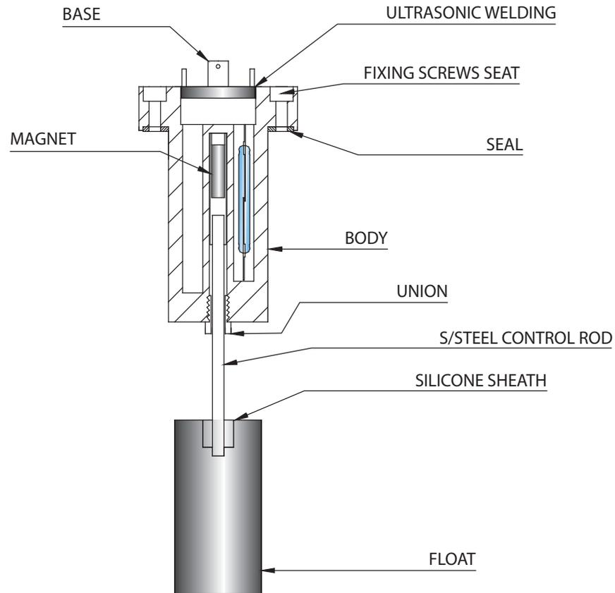
\* The required length can be obtained simply by cutting the steel rod, using an ordinary pipe cutter; or the switching point can be varied by using a float with through hole allowing the required liquid control point to be modified whenever necessary.
