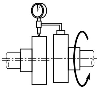
With the indicator set to zero, check the shaft alignment by rotating the shaft and recording the maximum and minimum reading on the dial indicator. This values' difference should not exceed the published value  $\Delta r$  for each type of coupling.
