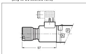
When the set screw is screwed and its point is aligned with the edge of the knob, tighten the knob till it touches the spool: in this position the override is not engaged and the valve is de-energized. After adjusting the override, tighten the set screw in order to avoid the knob loosing.
