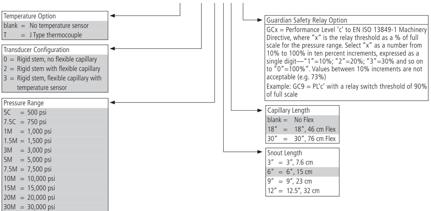
Standard mating connector Dynisco P/N 711600 or 6-pin mating connector cable assembly. Shaded sections refer to standard configurations. Accuracy may be affected if non-standard configurations are used. For additional options please consult factory.
