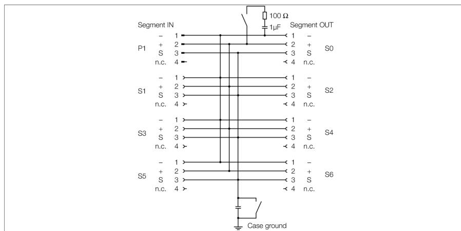
The 6-channel Ex junction box JBBS-49-E613/Ex is designed for FOUNDATION™ fieldbus systems.
